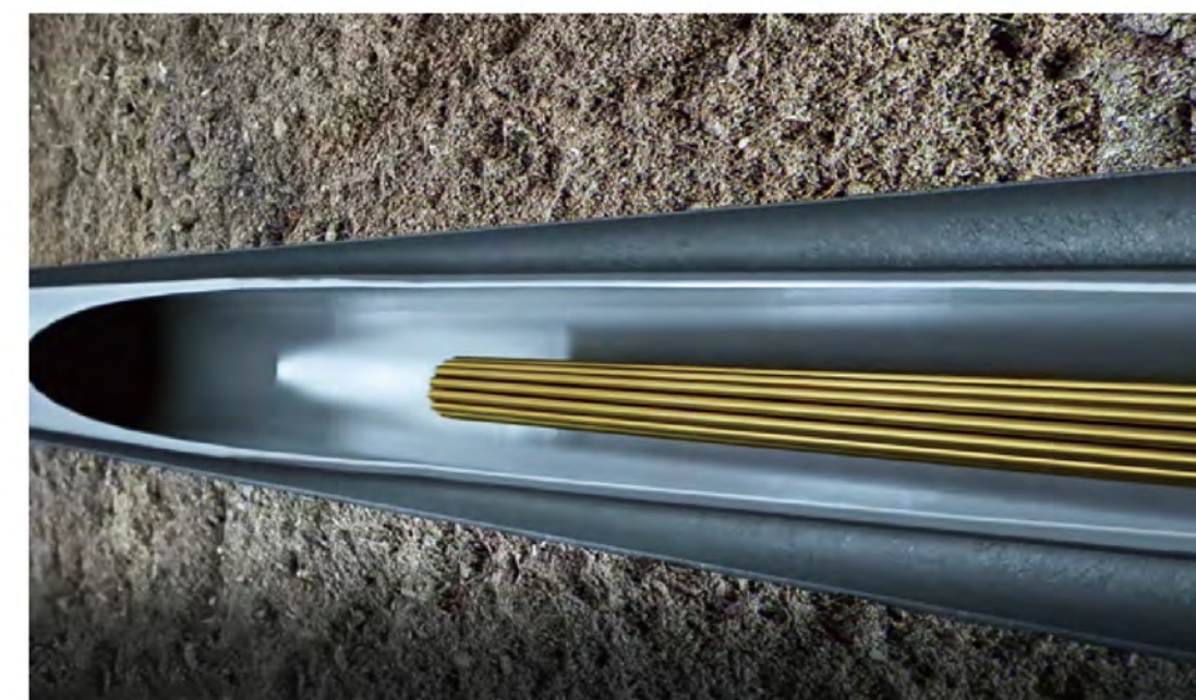
Fig.: Coiled Tubing Containing Logging Cable Injection
