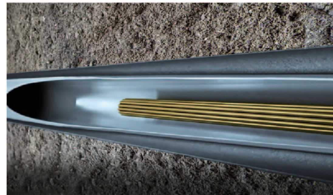
Fig.: Coiled Tubing Containing Logging Cable Injection
