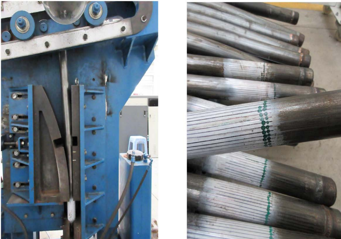
Figure 5—Fatigue Test Machine and 10 deg Rotation Samples
